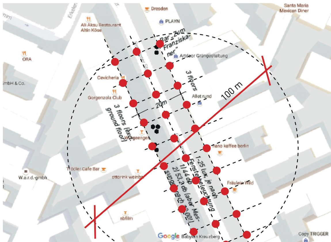
Fig. 5: exemplary grid for measurements in a 10m-grid.
